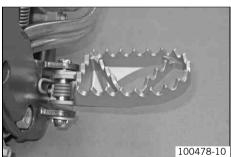
Mount the footrests with the springs and bolts. Secure the bolts using the washers and pins.
